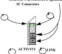
Note - to support long fiber distance with the Magnum 8000X, use either 10Mbps modules in front ports (which can go up to 2Km), or use a 100Mbps full-duplex SPM in the bonus port which has no collision domain limits.
